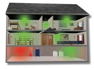
Smoke/fire is detected in one area of a home, the lamp will alarm with both strobing RED & WHITE light while audibly sounding the siren, giving notice of an immediate danger.
